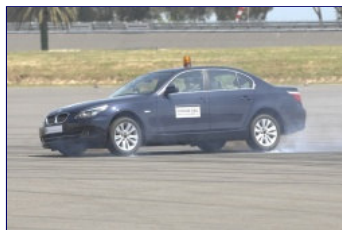
A driver demonstrates ESC in a BMW 5 Series. Click image to enlarge
